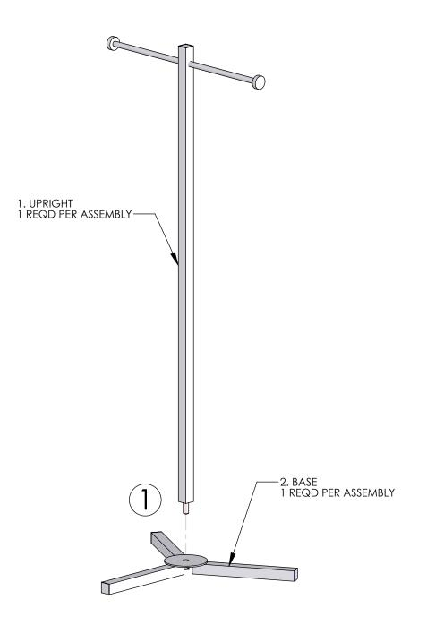
$\mathbbmspace{1}$  screw the upright into the threaded hole in the center of the base. Use the faceouts of the upright to help tighten.
