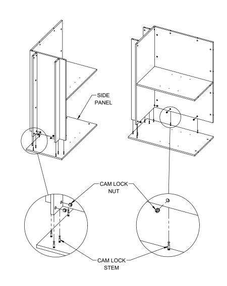
MOUNT THE OTHER SIDE PANEL TO THE REST OF THE UNIT USING (8) CAM LOCKS.
