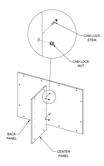
MOUNT BACK AND CENTER PANEL TO THE BASE PANEL USING (6) CAM LOCKS.
