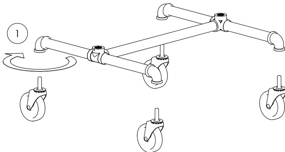
1 SCREW THE CASTERS INTO THE BASE AS SHOWN USING WRENCH
