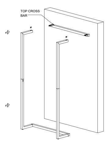
LIFT THE ASSEMBLED FRAME UP TO THE UPPER CROSS BAR MOUNTED ON THE WALL AND ASSEMBLE AS SHOWN WITH THE REMAINING COUNTER SUNK SCREWS.
